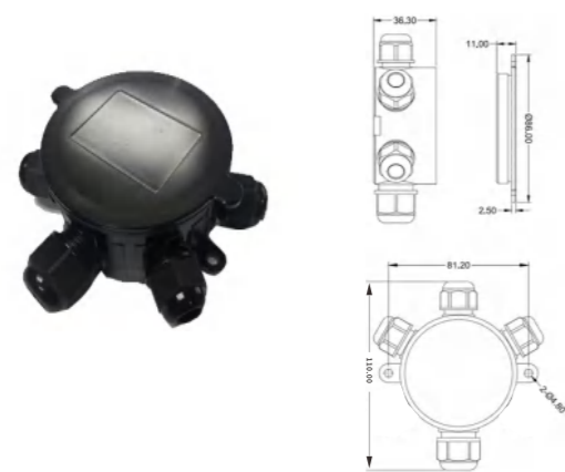
Name: Junction Box Model: EIP68-3A EIP68-3B EIP68-3C EIP68-3D Color: Black IP Rating: IP68 Waterproof depth: 4 m Weight: 65g Approval: ROHS
