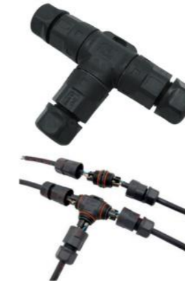
Parallel T type three way Waterproof plug connector 2P/4P Model: 3T Input: 300V max Rated Current: 13A IP Rating: IP67 Applicable Diameter of Cables: 5---9mm Insulator material: Nylon Connection: screw type
