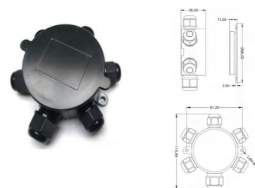
Name: Junction Box Model: EIP68-5A EIP68-5B EIP68-5C EIP68-5D Color: Black IP Rating: IP68 Waterproof depth: 4 m Weight: 78g Approval: ROHS
