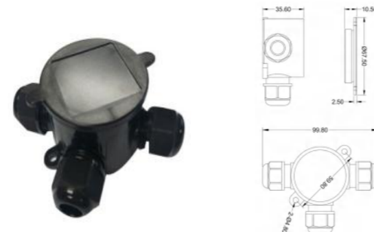
Name: Junction Box Model: EIP68-2A EIP68-2B EIP68-2C Color: Black IP Rating: IP68 Waterproof depth: 4 m Weight: 53g Approval: ROHS
